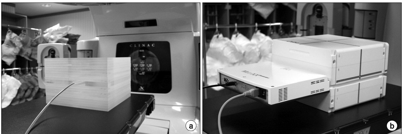
Fig. 2. Setup of quality assurance (a) point dose with polystyrene phantom and CC01 ion-chamber and (b) I'm MatriXX with Multicube phantom.
