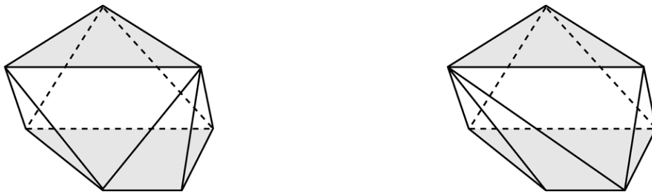
Figure 7. Stacked triangle and quadrangle with vertices connected either by short up-down edges, which yields almost regular triangular surfaces (left) or by long up-down edges, which doesn't (right).
