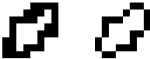
Figure 2. A contour with one or two pixel lines (left), which is converted into a contour with one pixel line (right).
