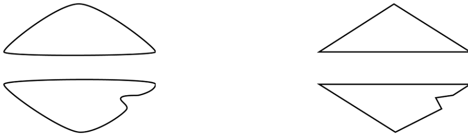
Figure 5. Stacked two contours (left), which are converted into two polygons composed of vertices and edges (right).
