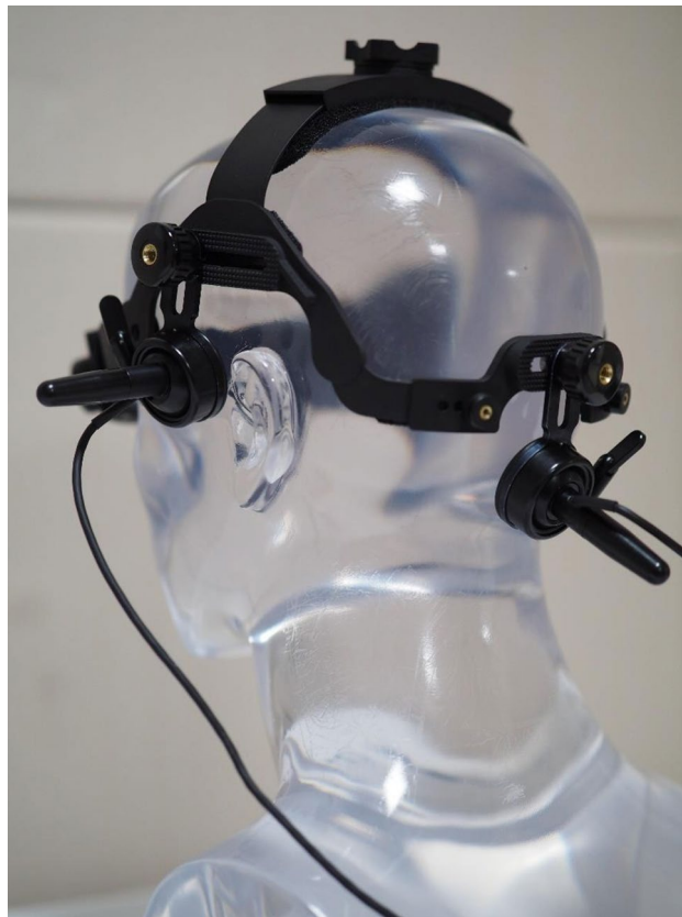
Figure 3. Fixable device which can be placed on the MCA and BA during TCD of the PFO.
